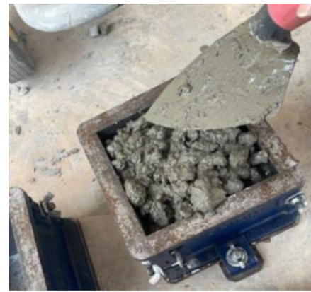
Fig. 4. Casting Concrete Cubes
