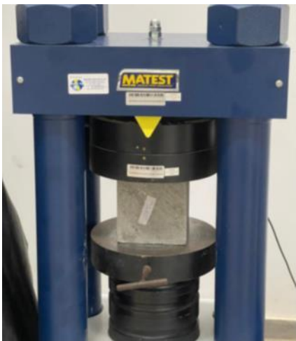
Fig. 6. Compressive Strength Testing Machine
