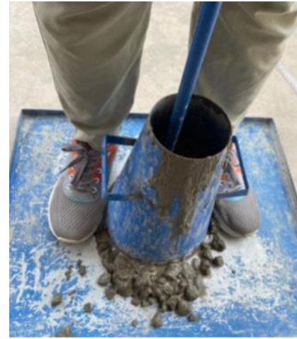
Fig. 9. Performing Slump test
