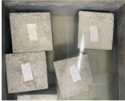
Fig. 5. Curing Concrete Cubes
