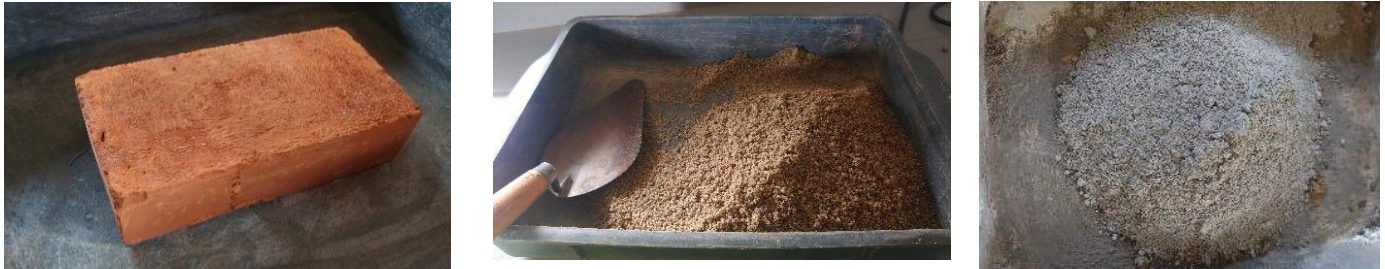
Fig 01: Material components: (a) Clay bricks, (b) Sand preparation, (c) Cement mortar mixing.
