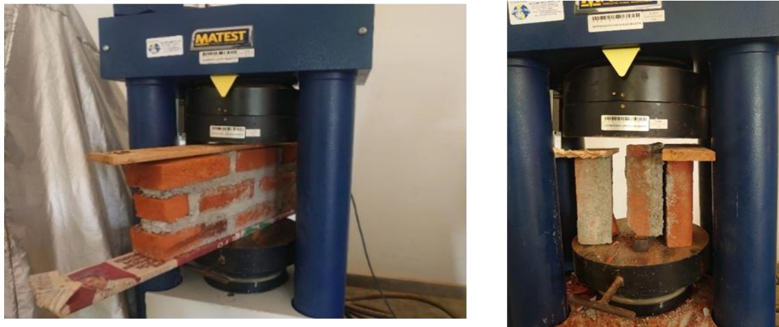
Fig 3. Experimental setup: (a) Compressive strength testing apparatus, (b) Shear strength testing configuration.
