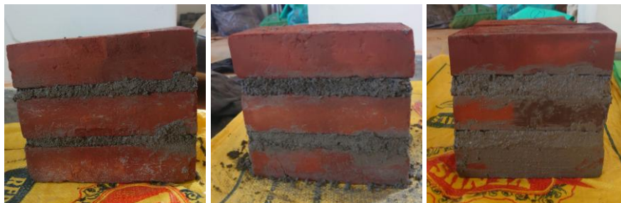
Fig 02. Wall construction process shows different joint thicknesses: (a) 10 mm joints, (b) 20 mm joints, (c) 30 mm joints.
