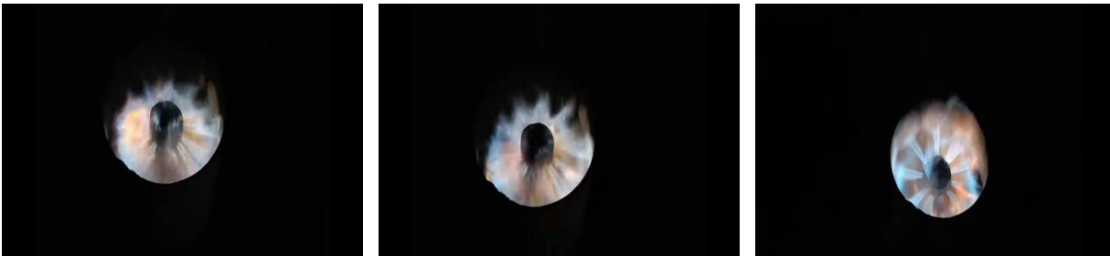
Fig 8 Effect of primary air pressure on flame visual observation of LDO
