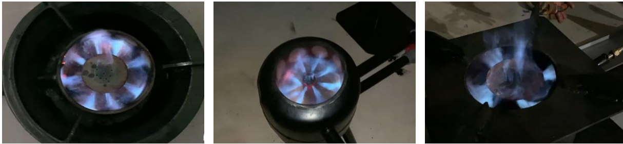
Fig 7 Effect of primary air pressure on flame visual observation of WCO
