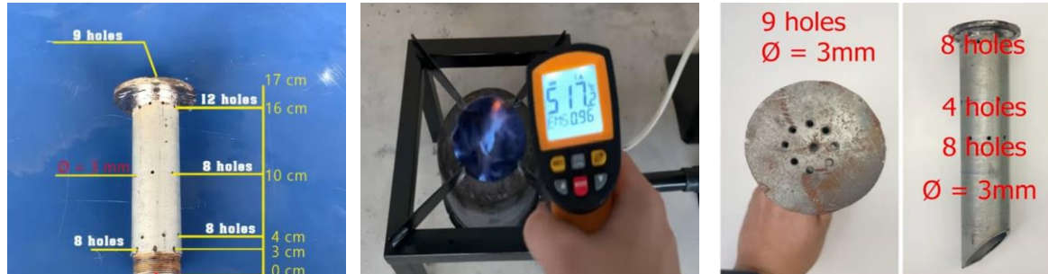
Fig. 1 Experimental design of the burner
