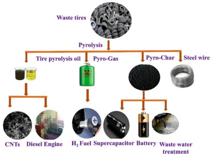
Fig. 5. waste tire pyrolysis products and their applications [42]
