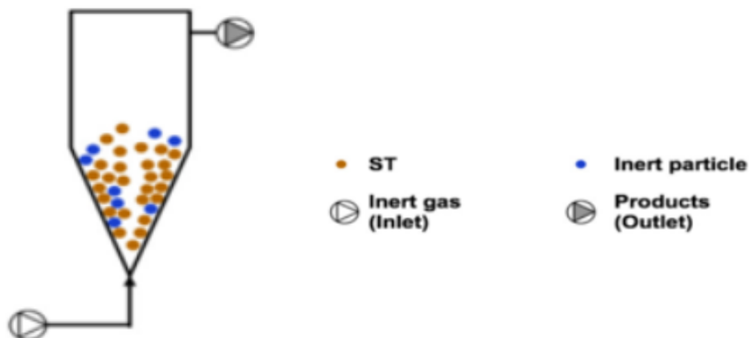
Fig. 17. Diagram of a SCBR reactor [59]
