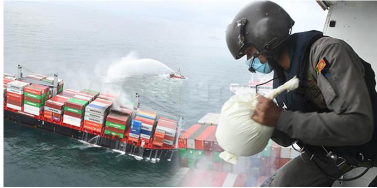
Figure 03: Dry chemical powders are also dropped over the vessel[11]
