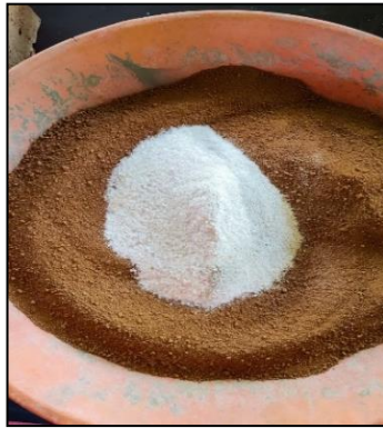
Fig. 1:- Addition of sieved glass powder to cleaned & weathered clay
