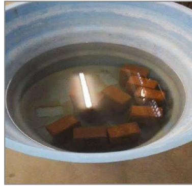
Fig. 7:- Water absorption potential estimation
