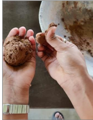
Fig. 3:- Smearing test conduction
