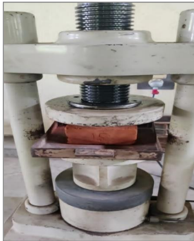
Fig. 6:- Compression strength estimation
