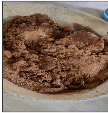
Fig. 2:- Initiation of tempering process to form the lump for moulding
