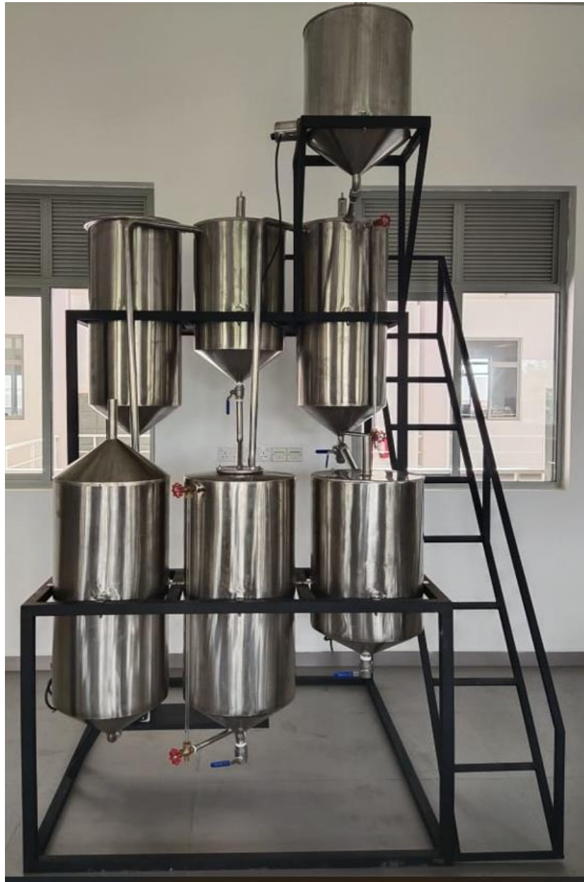
Fig. 8. Biodiesel production Pilot plant at the laboratory
