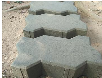
Fig. 6. Stacked in the Brickyard for Air Drying – Side View
