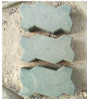
Fig. 7. Stacked in the Brickyard for Air Drying – Plan View
