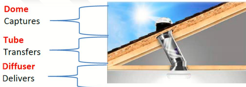
Fig. 4. Structure of a Solatube [8]
