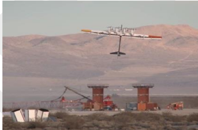
Fig.02.The crosswind device with On-Board Generation [7]
