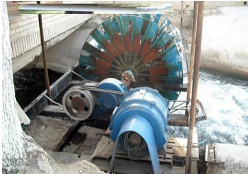
Fig. 02. The rainwater converting into the electricity Pico hydropower system [18]
