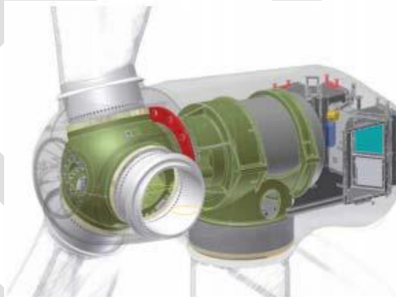
Fig. 17. The 10MW HTS wind turbine generator [38]
