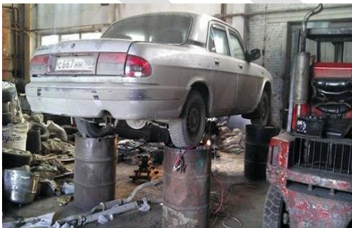
Fig. 1 Unsafe method used in small scale repair centers
