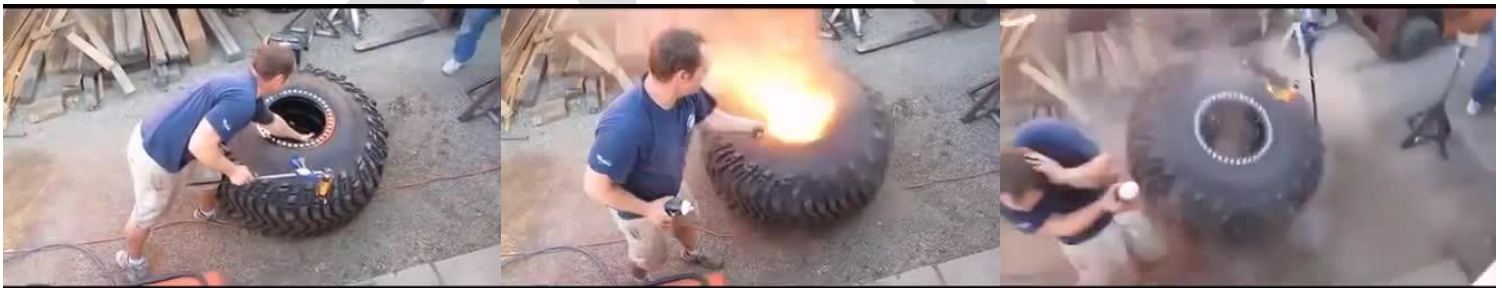
Fig. 4. Truck tire bursting during repair
